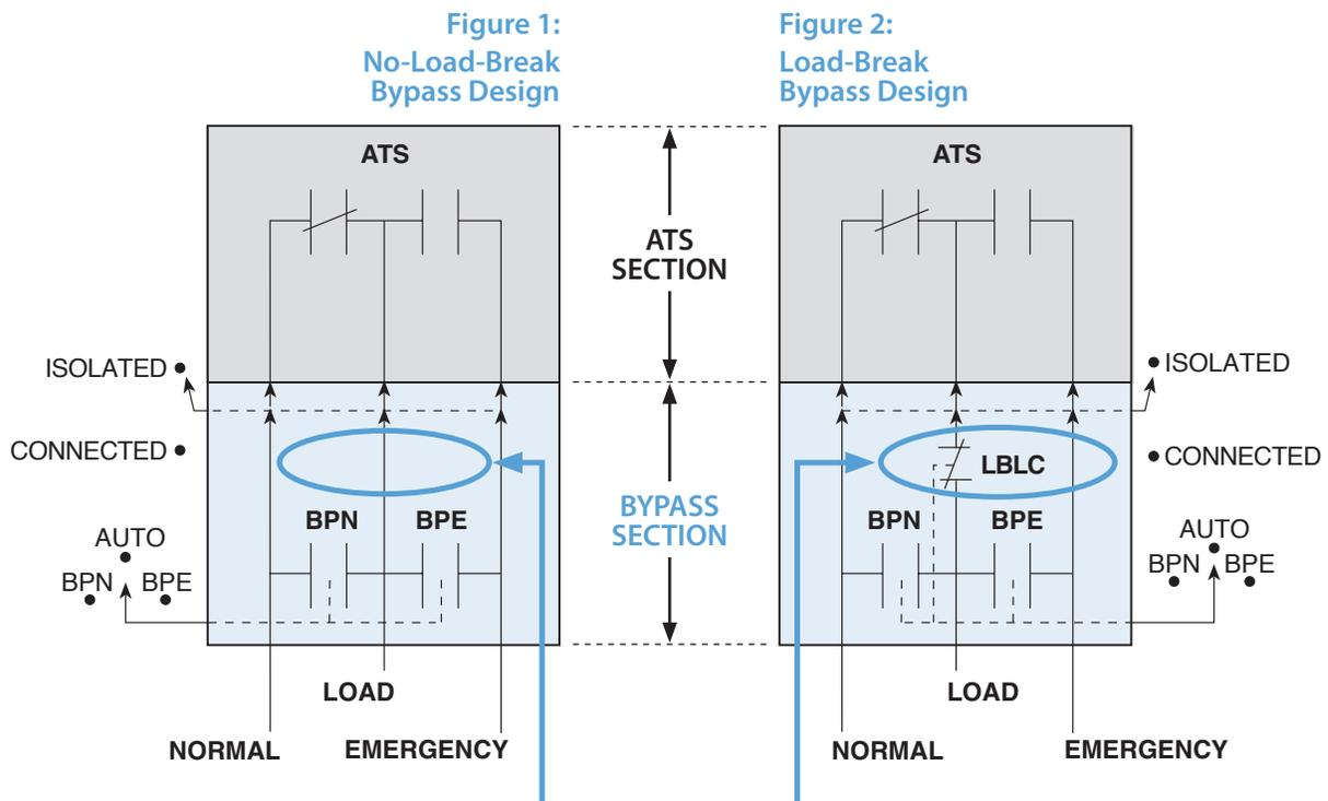
As shown above, competitors' designs do not have any load contacts. Russelectric's design has overlapping load contacts (not shown), however, both designs add steps and time, and limit the operator's options in an emergency situation.
